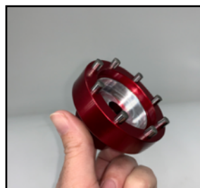
A. Hub nut tool (This tool requires the axle to be removed for wheel bearing service)
