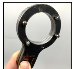
B. Hub nut tool does not require axle to be removed.
