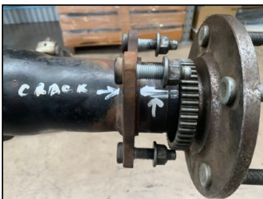
Common failure for RAM 1500 wheel bearing area
