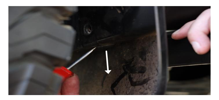
STEP 3: Align OTA 35" Tyre Mudflap to mounting points on the inner guard - Once aligned correctly, trace around the top edge with a marker pen to create a clear and visible line to cut.
