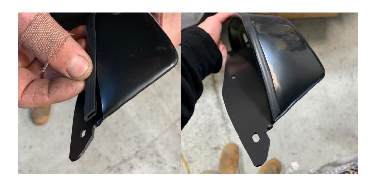
STEP 3: (Door flare only) Remove one of the body clips from the OE door flare and insert into the mount located on the inside of the OTA door flare.
