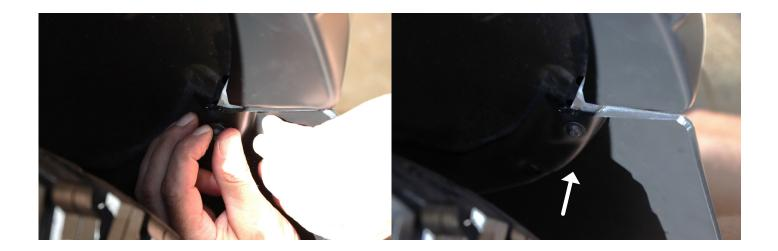
STEP 2: Push and insert the clip into the hole
