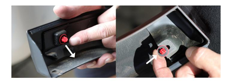
STEP 4: (Door flare only) Carefully align the flare to the OE mounting point at the bottom of the flare and fit 1 small OE clip.
