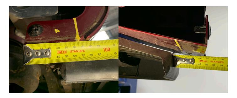
STEP 6: Using the Multi-Tool again, carefully cut along the marked lines to remove the piece of skirting.
