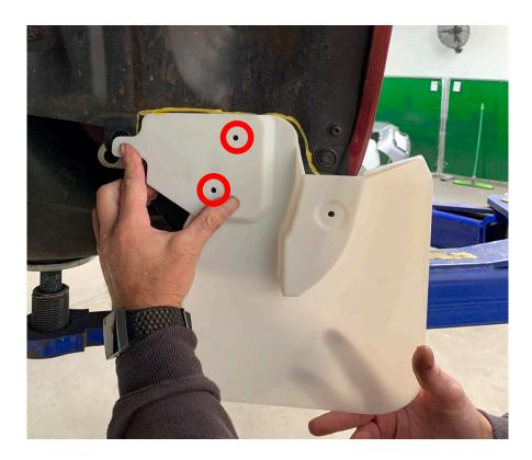
STEP 8: Using a 4mm Drill Bit, Pre-drill the the marked holes on the crash tube. Once pre-drilled, realign the mudflap and insert the two supplied self tapping screws. The OTA 35" Mudflap, should now be installed.
