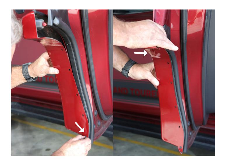
STEP 5: Using the remaining 2 small OE clips, aling holes and insert into the mounting hole in the corner and the top of the flare.
