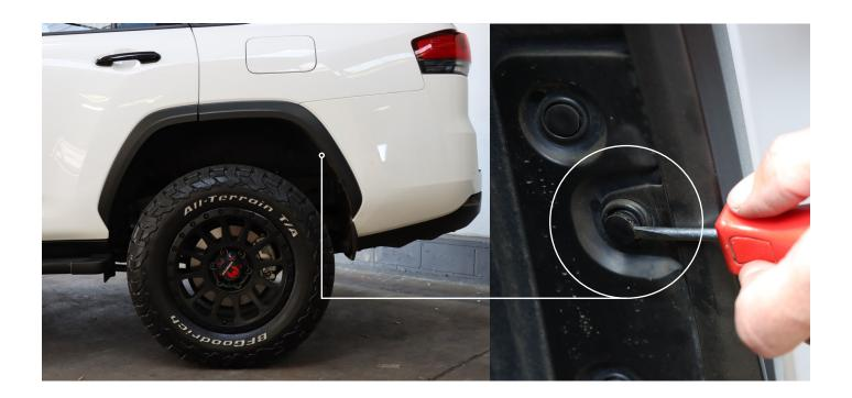
STEP 4: Beginning with the door flares, carefully grip and pull the flare off the body of the car. Work your way along until you have removed 5 clips, which will release the flare.
