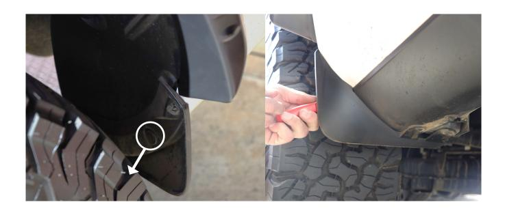
STEP 2: Using the 4mm Allen key, remove the 3 screws from the mudflap. (1 on the front face and 2 at the rear, under the car)
