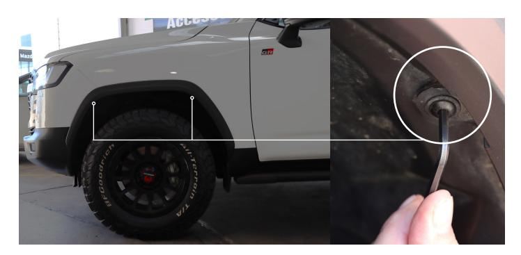
STEP 4: Starting from the rear of the front flare, carefully grip and pull the flare off the body of the car. Work your way along until you have removed 11 clips.
