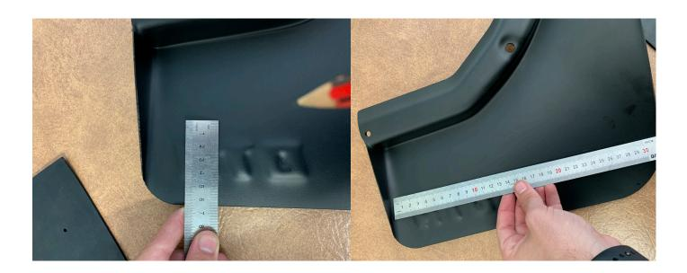
STEP 2: Align the supplied rubber piece with the marked line and outer edge of the mudflap and mark the 3x Mounting holes. (Check mounting holes to ensure they are correctly marked)
