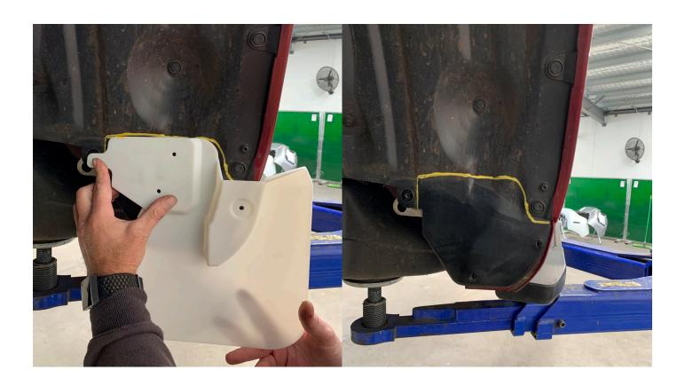
STEP 4: Using a Multi-tool with a cutting blade/edge, carefully trim along the line as marked, ensuring not the cut further than the thickness of the inner guard. Once comepletey cut, this will remove the cut piece of inner guard and expose the Aluminium crash tube, which will be used for mounting.
