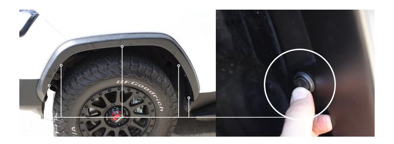
STEP 5: After refitting the clips, put the two supplied spacers between the flare and hole, screw in the two remaining screws to complete the fitment of your front flare.
