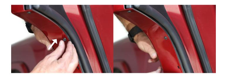
STEP 6: Using the OE screw, finger tighten into the mounting hole and fully secure with a 4mm Allen key.
