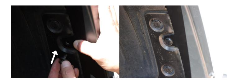
STEP 9: Secure the rear flare using the remaining the OE screw. Finger tighten, then fully secure using the 4mm Allen key.
