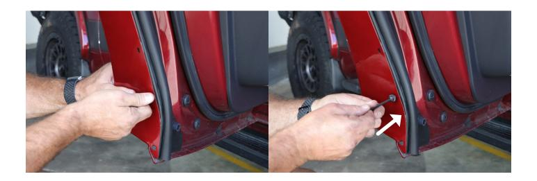
STEP 7: Firmly press the flare against the car and using a 3mm drill bit, pilot drill in the centre of the remaining 2 slots. Once drilled, screw in one of the supplied torx bit screws with the T20 wrench.
